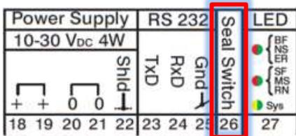
Setup or changes of calibration can only be performed with an open seal switch (26). Changes lead to get a new TAC value, increased by +1.
