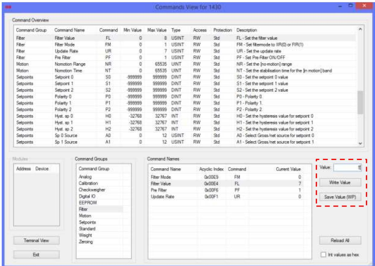
24. Change Decimal Point setting via button Calibrate Enable – see below.
