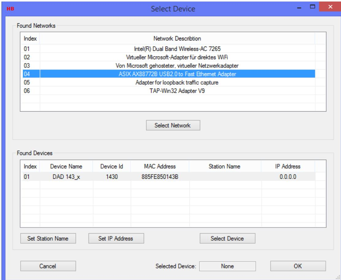
12. Now you see the found device(s), which are connected via Ethernet based Port 1 or 2:
