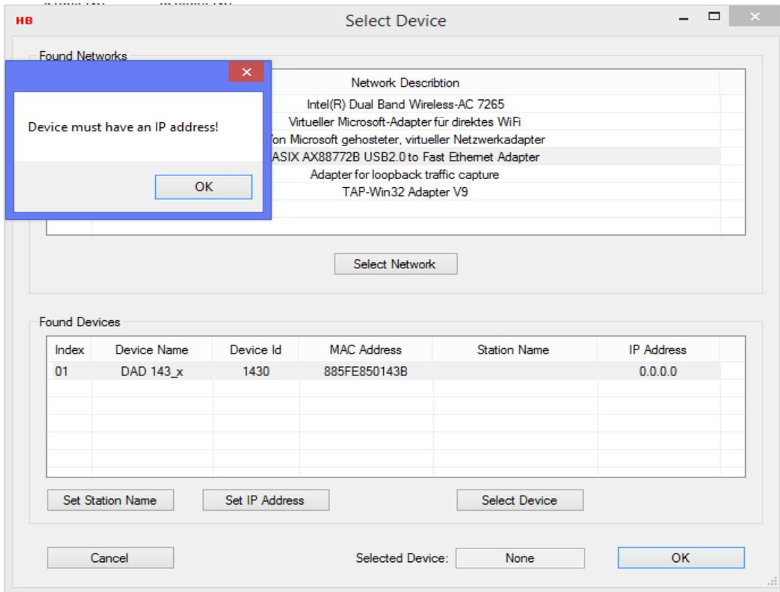
**Note:** The reason for this message is that Index 01 shows a device, which has no **Station Name** and no **IP Address**.
