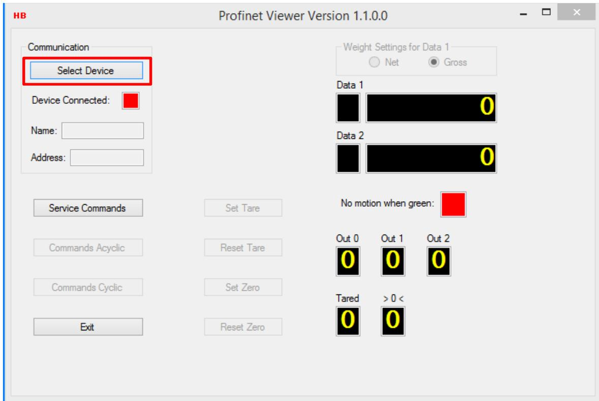
2. Press button 'Select Device' in the upper window to check if the **Npcap driver** is installed on your PC. If you get the error message like the one below, the driver is not installed.
