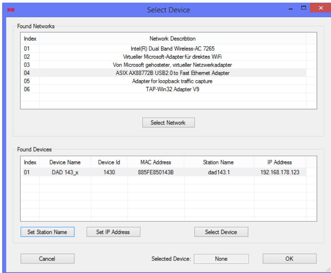
19. Mark Index 01 and press the button OK to start ProfiNet communication.
