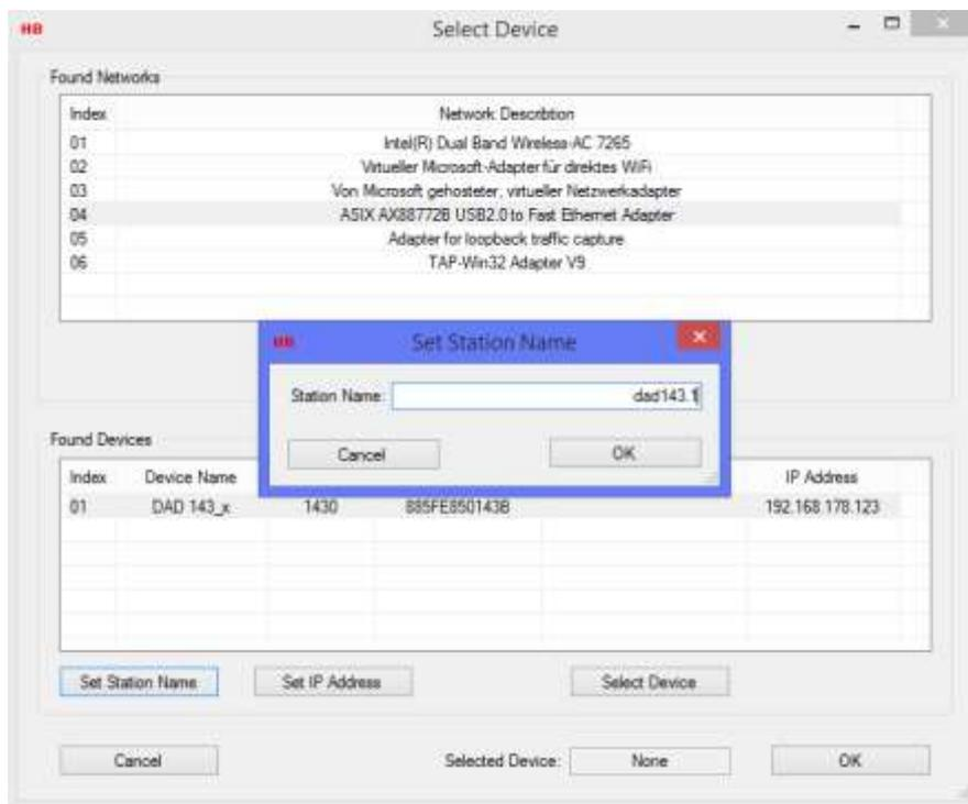
18. The procedure Set the Station Name and IP Address is finished now.
