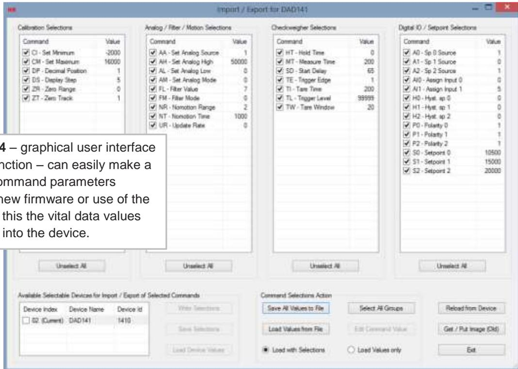
The Software **DOP4** – graphical user interface with oscilloscope function – can easily make a backup of all vital command parameters before download a new firmware or use of the FD command. After this the vital data values can be loaded back into the device.
