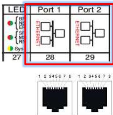
The two RJ45 Ethernet ports (28 & 29) are connected to an internal switch. The Ethernet ports support 10BASE-T and 100BASE-TX. Half-, Full- and auto negotiated duplex mode. MDI, MDI-X and Auto-MDIX crossover control.
