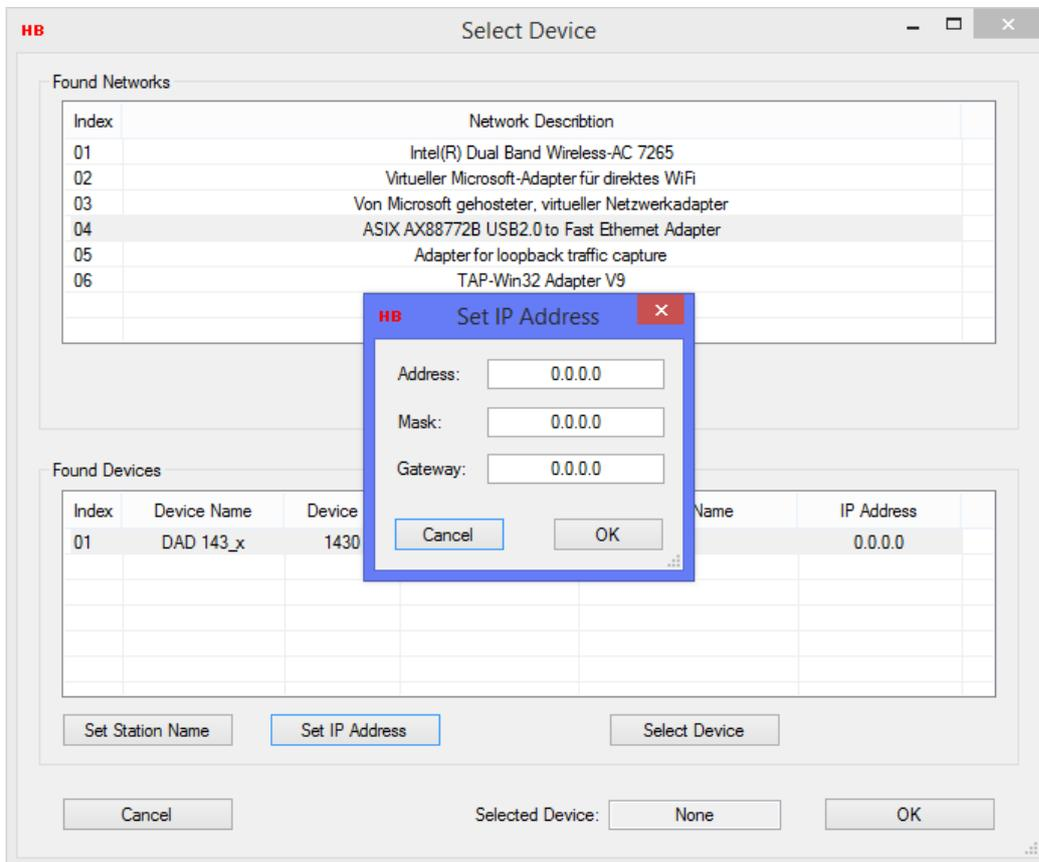
14. In any case you have to set Address and Mask. The Address range, e.g. 192.168.178.xxx, must be adjusted to your network. The xxx you can choose freely. Network Mask set to 255.255.255.0. A Gateway Address is not required.
